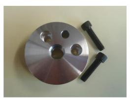
You are now ready to fit a spin-on oil filter to your Austin Healey. We recommend a Crosland 357 or similar high quality filter. Always grease the sealing ring of the filter before fitting as this helps to remove it later. Always check for oil leaks on initial start-up. Observe the original filter change intervals. Never tighten a spin-on filter with a filter removal tool.
